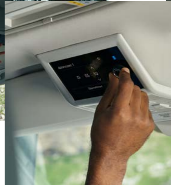
The auxiliary heater can be set to continuous operation for the night on the new Camper control unit.
